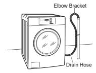
3 Use a tie strap to secure the drain hose in place.
